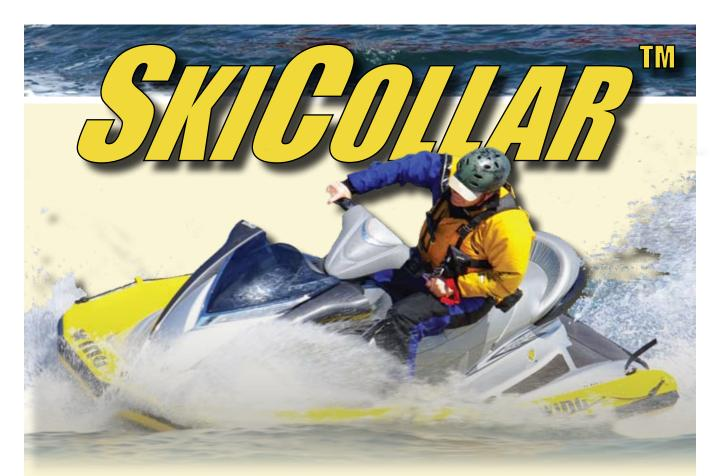
The SkiCollar<sup>™</sup> is an ultra durable inflatable tube that can be easily affixed to many PWC hulls to improve lateral stability, afford shock absorption and provide additional flotation. It installs quickly to the craft without hardware or tools, greatly improving PWC stability without sacrificing exhilarating speed and tight turning capabilities. Applications range from rescue/patrol, protection for rental units, or simply training wheels for novice riders.
